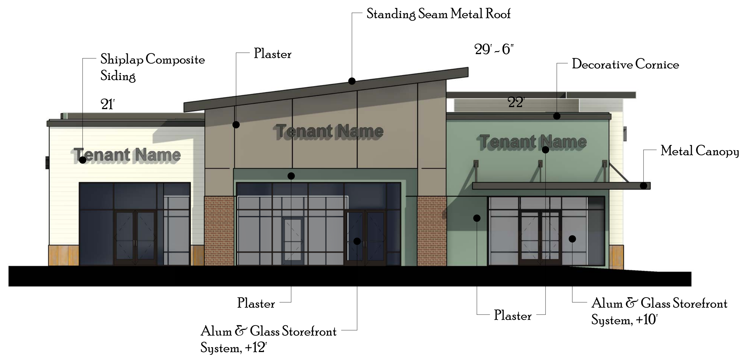
East Elevation ~ Pad 2
