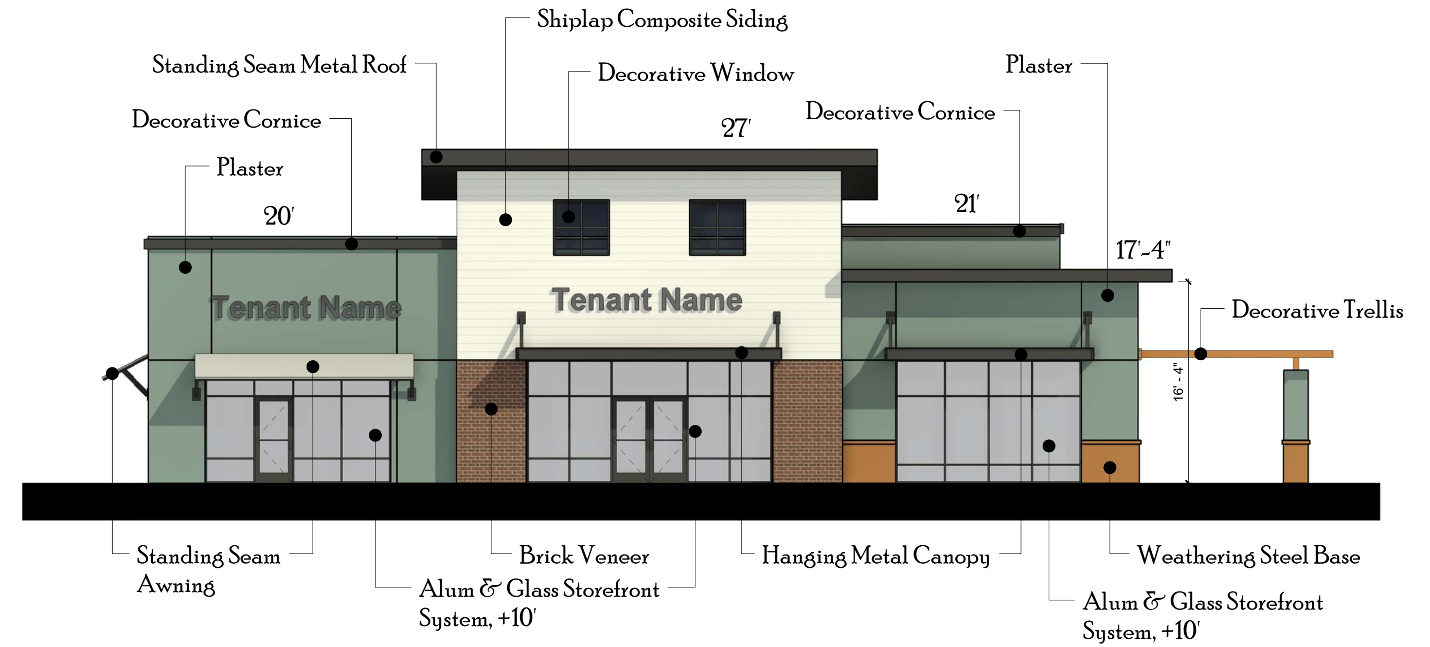
North Elevation ~ Pad 3
