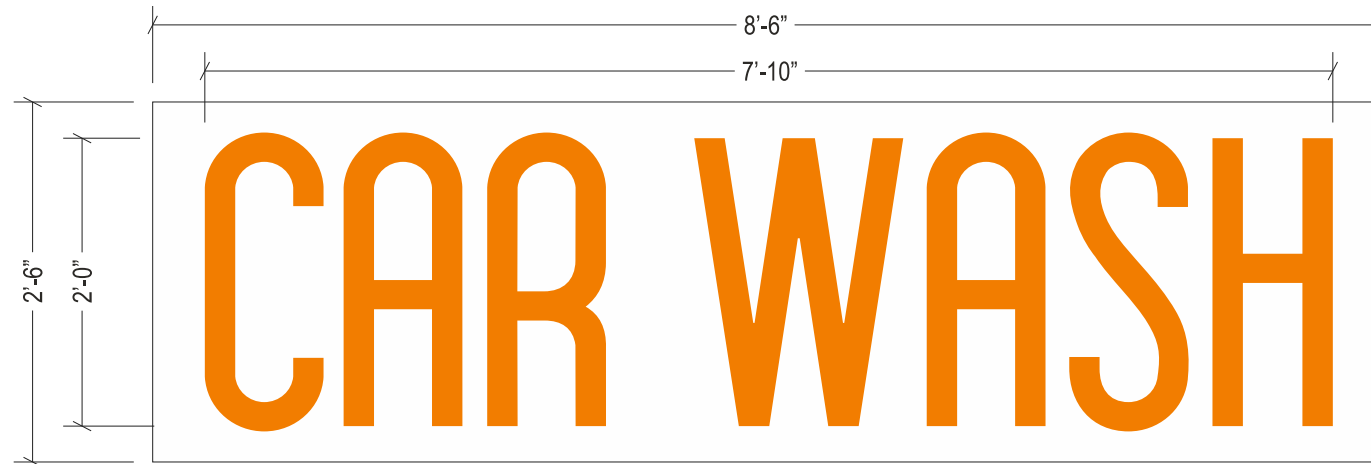
SIGN B: LED ILLUMINATED FACE/HALO LIT PCL ON PAN BACKGROUND Scale: 3/4" = 1'-0"
