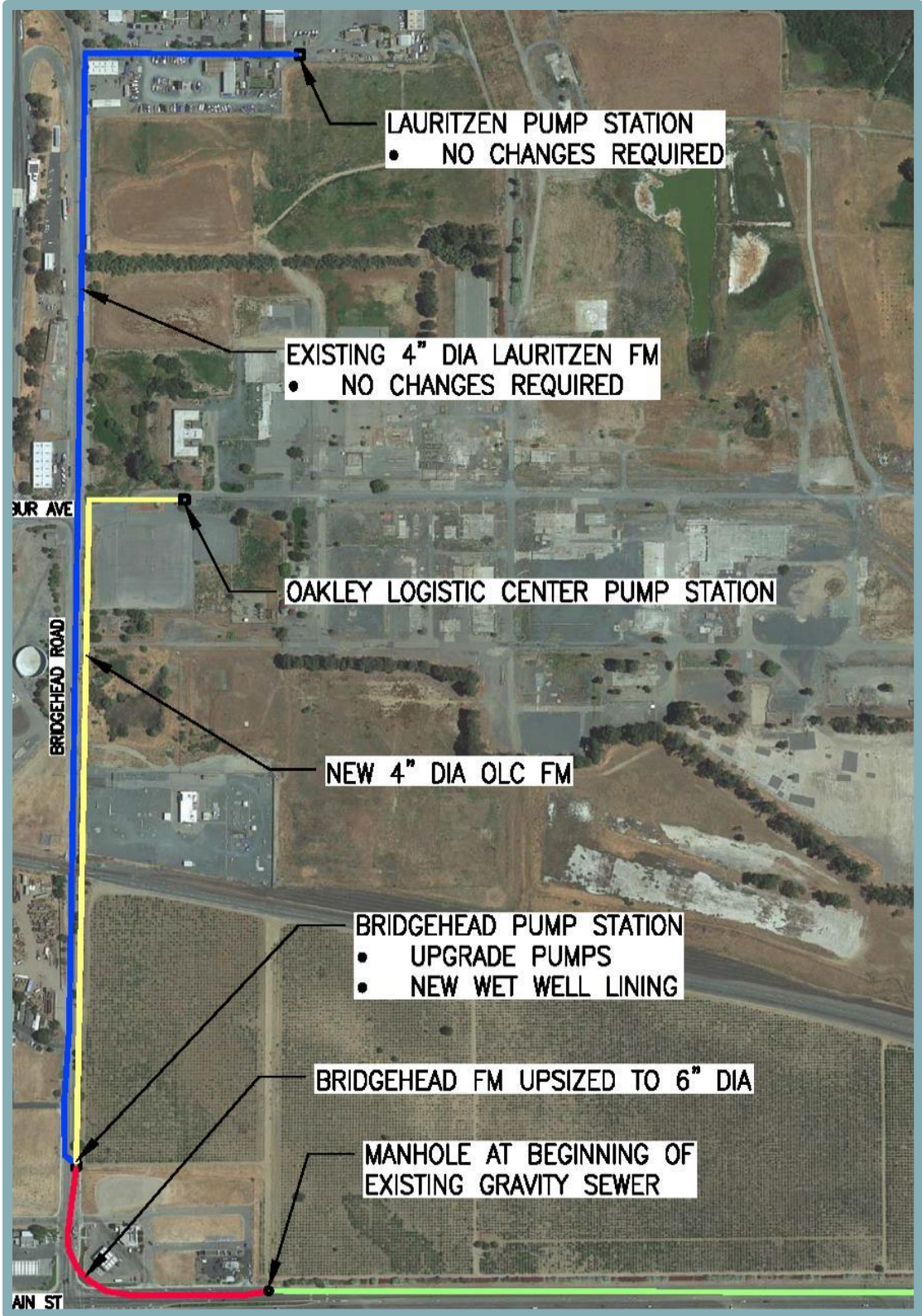
Figure 4.5-1 Proposed Sewer Improvements
