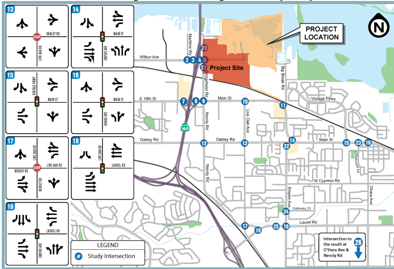
Figure 4.4-3 Lane Configurations – Existing Conditions (2 of 3)
