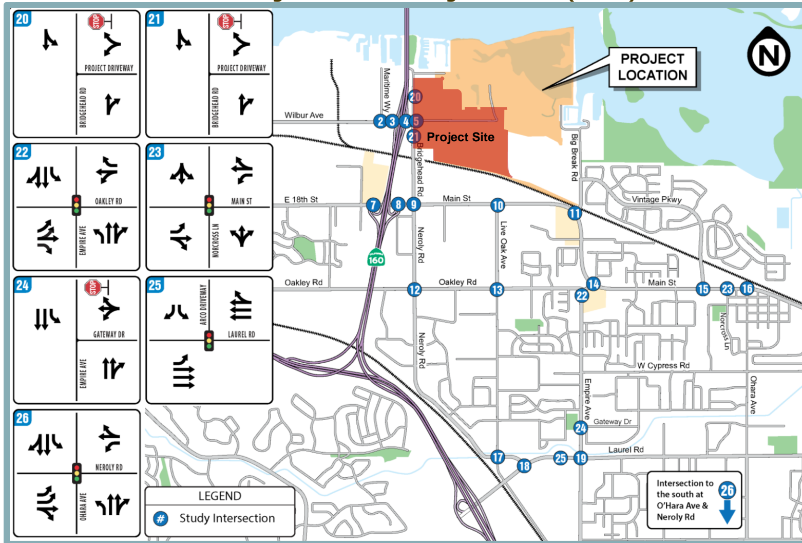
Figure 4.4-4 Lane Configurations – Existing Conditions (3 of 3)
