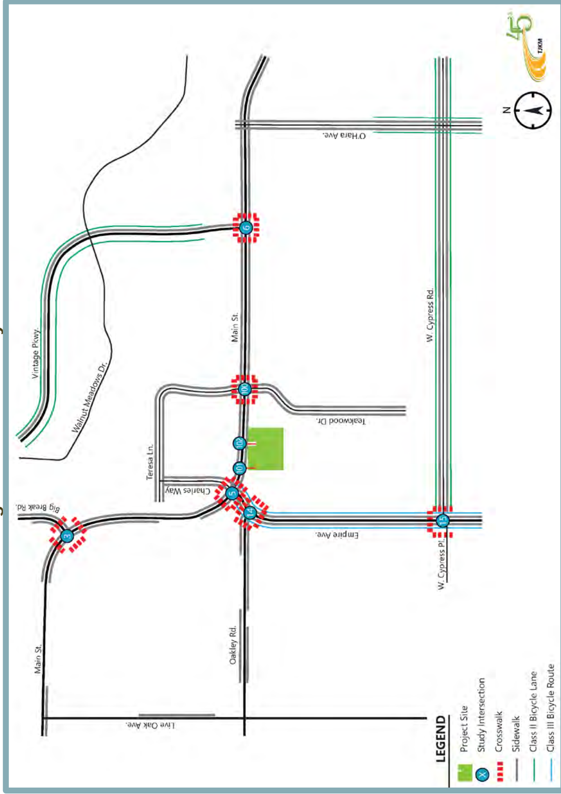
Figure 12 Existing Pedestrian and Bicycle Facilities
