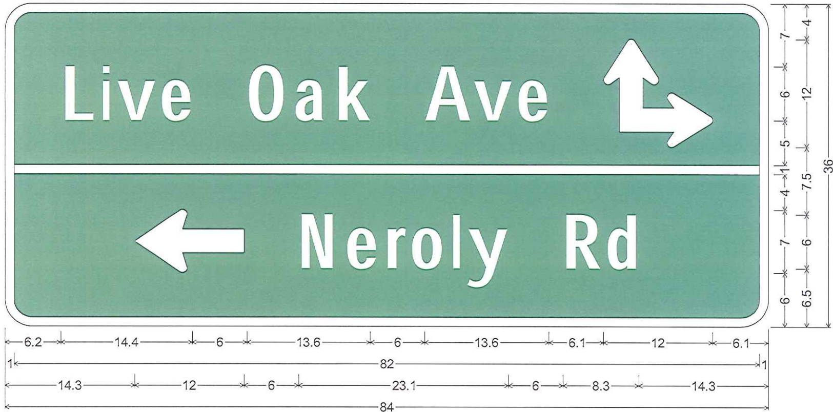
Sign 2; 3.0" Radius, 1.0" Border, White on Green; "Live Oak Ave" D 2K; 90 Deg Double Headed Arrow Custom 12.0" X 12.0"; Standard Arrow Custom 12.0" X 7.0" 180°; "Neroly Rd" D 2K;
