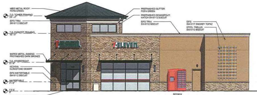
1 EAST ELEVATION (HOWE WAY) 3/16" = 1'-0"
