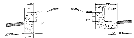
CURB DETAIL NO SCALE CURB & GUTTER DETAIL NO SCALE
