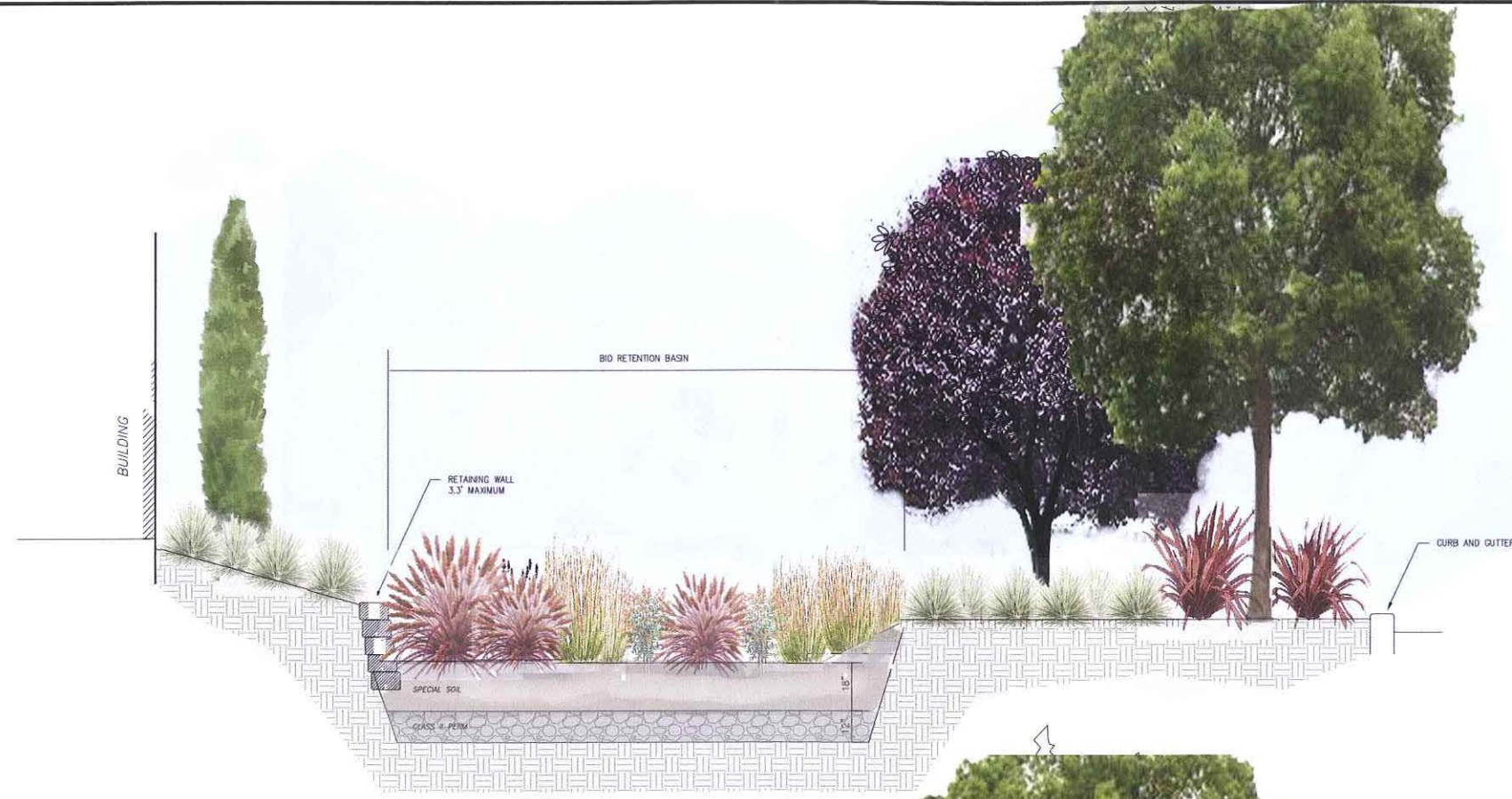
BIO-SWALE SECTION A-A
