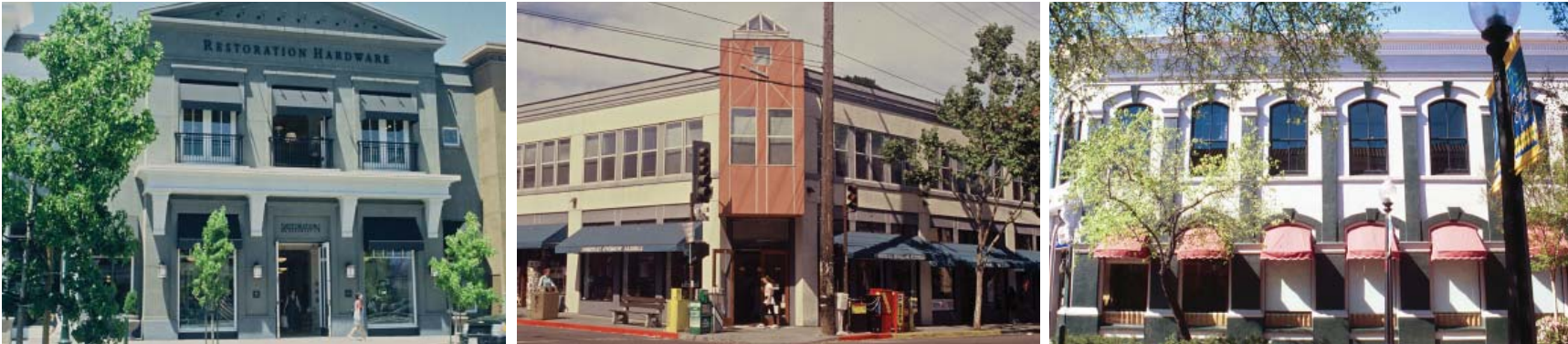
Door and window openings should be aligned and composed vertically. In general, first floor windows should be larger than upper floor windows.
