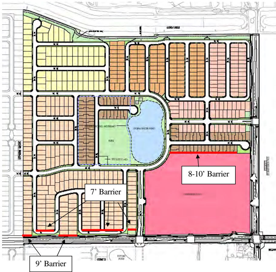
Figure 2: Preliminary Barrier Design
